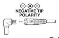
For devices with positive polarity ( ), the DC adaptor must be connected with the positive symbol position in front of the word "TIP".
