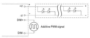
"DO NOT connect "DIM- to -V"
