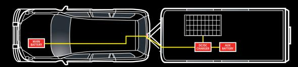
Combines your solar and vehicle's power to deliver a 3 Stage charge ensuring longer battery life and performance
