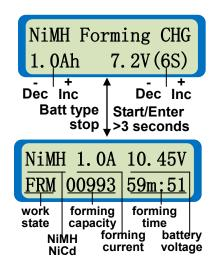
The left side of the first line shows the type of battery (NiCd/NiMH). The value on the left side of second line sets the cell capacity and the value on the right side of second line sets the cell count and nominal voltage of the battery pack. Press **Start/Enter** for more than 3 seconds to start charging.
