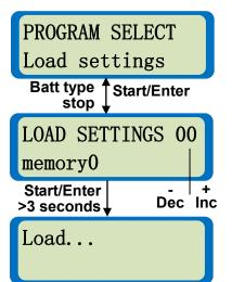
This screen displays the data load program. You can press Inc▶ & Start/Enter button for 3 seconds to enter this interface directly.
