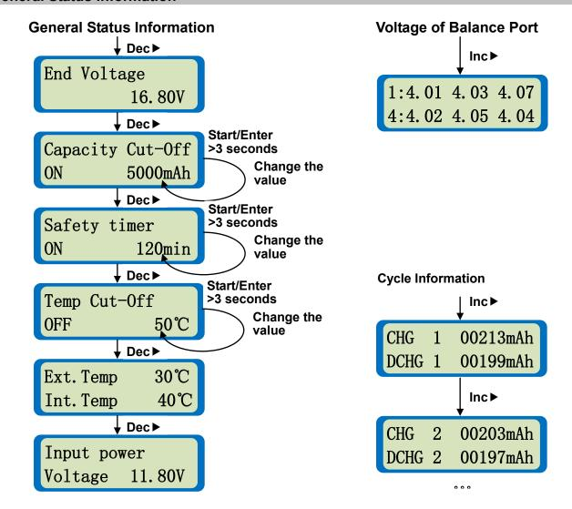
**Note:** Toggle back to the last viewed parameter via the **◄Dec** button, press **◄Dec** again to move to the next parameter.
