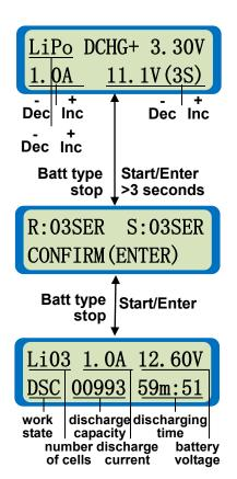
Discharge Lithium battery. The left side of the first line set the type of battery (LiPo, Lilo or LiFe) and the value on the right side shows the final discharge voltage of each cell. The value on the left side of second line sets the charge current and the value on the right side of second line sets the cell count and voltage of the battery pack. After setting the current and voltage, press **Start/Enter** for more than 3 seconds to start the next process.
