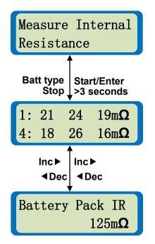
Measure internal resistance. You can press **Start/Enter** for more than 3 seconds to start the process and stop at any time by pressing **Batt type/Stop.**
