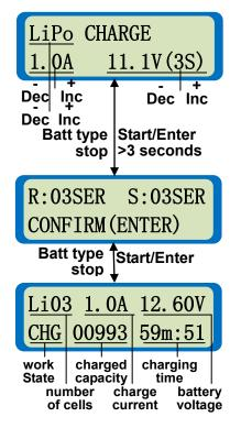
The left side of the first line set the type of battery (LiPo, Lilo or LiFe). The value on the left side of second line sets the charge current and the value on the right side of second line sets the cell count and voltage of the battery pack. After setting the current and voltage, press **Start/Enter** for more than 3 seconds to start the next process.
