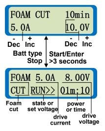
The value on the right side of the first line sets the run duration in minutes. The second line shows the upper limit of current on the left and foam cut voltage on the right. After setting the current and voltage press **Start/Enter** for more than 3 seconds to start the process. A beep tone will sound. Runing time: 0– 90 min (0 refers to stopping the process by yourself) Current: 0.05 – 10A, voltage: 1 – 25V
