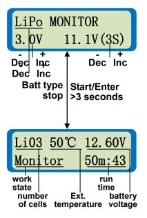
Monitor mode of Lithium battery. The left side of the first line sets the type of battery (LiPo, Lilo or LiFe). The value on the right side of the second line sets the low limit of voltage and the battery pack number. After setting the current and voltage press **Start/Enter** button for more than 3 seconds with a sound "Di" to start the next process.
