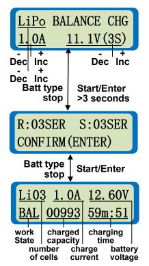
Balance charging mode of Lithium battery. The left side of the first line set the type of battery (LiPo, Lilo or LiFe). The value on the left side of second line sets the charge current and the value on the right side of second line sets the cell count and voltage of the battery pack. After setting the current and voltage, press **Start/Enter** for more than 3 seconds to start the next process.
