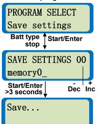
This screen displays the data save program. You can press **◀Dec** & **Start/Enter** button for 3 seconds to enter this interface directly.
