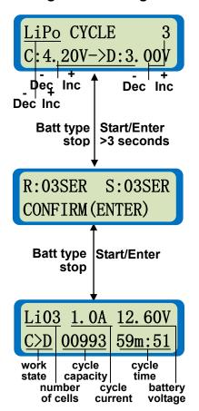
Charging/discharging cycle mode of Lithium battery.
