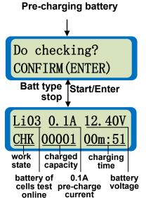
The following screen is displayed when the charger detects the battery voltage to be too low in the Normal charge or Fast charge modes.
