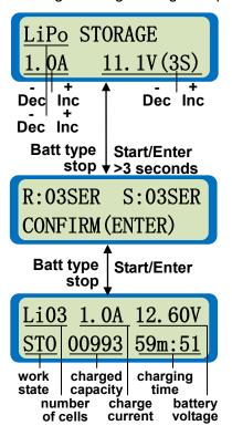
Storage of Lithium battery. The left side of the first line set the type of battery (LiPo, Lilo or LiFe). The value on the left side of second line sets the charge/discharge current and the value on the right side of second line sets the cell count and voltage of the battery pack. After setting the current and voltage, press **Start/Enter** for more than 3 seconds to start the next process.
