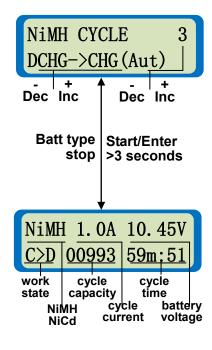
The left side of the first line shows the type of battery (NiCd/NiMH) and the right shows the cycle number. The second line shows the cycle direction you selected: (CHG (xxx) ->DCHG) or DCHG->CHG(xxx)). You can set the charge mode as "Charge Auto" or "Charge Manual". The discharge parameters are those set in NiCd/NiMH discharge screen. Press **Start/Enter** for more than 3 seconds to start the cycling.
