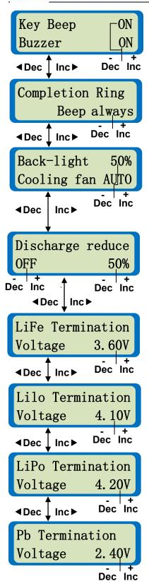
Key confirmation and alert tone. If the keyboard sound is ON there will be a beep when you press any key. If the buzzer is ON the **iCharger** will generate an alert tone for certain events.
