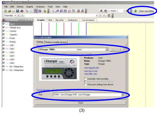
4) Start **iCharger**'s charge or discharge mode, then click "Start recording" to record data. See other functions of this software on "Help".
