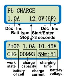
Charge Pb battery. The left side of the first line shows the type of battery(Pb). The second line shows the charge current and number of cells you selected. After setting the current and voltage press **Start/Enter** for more than 3 seconds to start the charging.
