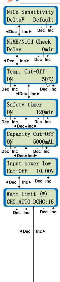
Usually, the NiCd battery voltage will drop a little right after reaching full charge. This is known as  $-\triangle V$ . You can alter the **iCharger**'s delta-peak detection sensitivity.
