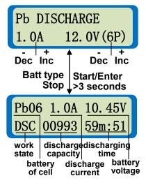
Discharging Pb battery. The left side of the first line shows the type of battery(Pb). The second line shows the charge current on the left and number of cells on the right. After setting the current and voltage press **Start/Enter** for more than 3 seconds to start the discharging.
