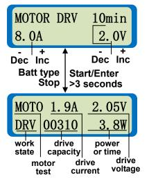
The value on the right side of the first line sets the test duration in minutes. The second line shows the upper limit of current on the left and drive voltage on the right. After setting the current and voltage press **Start/Enter** for more than 3 seconds to start the next process. A beep tone will sound.
