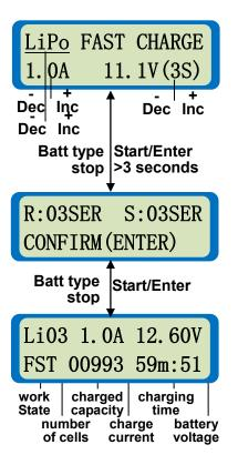
The fast charging mode of Lithium battery. The left side of the first line set the type of battery (LiPo, Lilo or LiFe). The value on the left side of second line sets the charge current and the value on the right side of second line sets the cell count and voltage of the battery pack. After setting the current and voltage, press **Start/Enter** for more than 3 seconds to start the next process.
