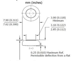
0.03 (0.001) Minimum Ref. (applies to top edge of gasket or edge of crimp, whichever is higher)
