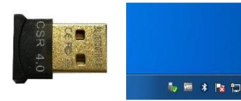
After searching, the bluetooth device will show and the last 3 bit 001 of name represent address code of digital power supply.
