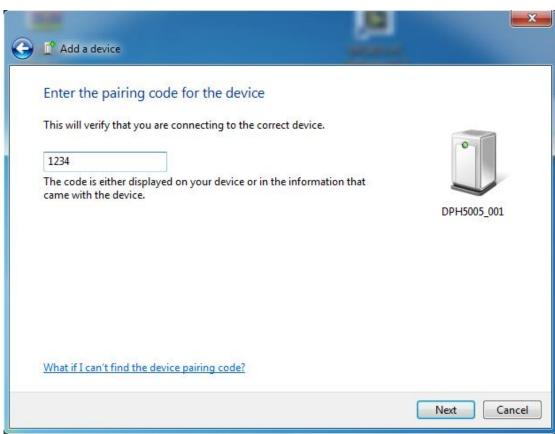
After connecting, the system will download and install Virtual serial port driver of bluetooth automatically. The smaller number CMO is what we use, eg COM3, we need to choose COM3 on upper computer.
