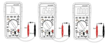
D) Connect the RED test lead to the positive pole of the tested diode, BLACK test lead to the negative pole. E) Read the present test result from LCD.
