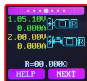
Data Connection Cable Impedance Measurement Interface
