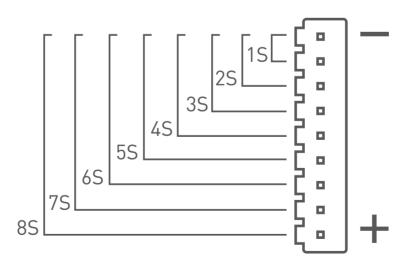
This product is suitable for the lithium battery which has the XH 2.54 balance port, connect the balance port align from BAT- as showed in the figure. When connecting 1S battery, input Voltage from XT60i must be more than 5V.
