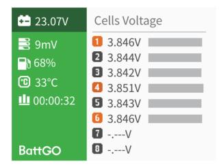
In balancing cells would show as yellow, and breath light is green during operation.
