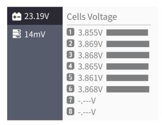
When battery connecting to balance port, BG-8S will show total battery voltage, max voltage difference between each cell and each cell voltage
